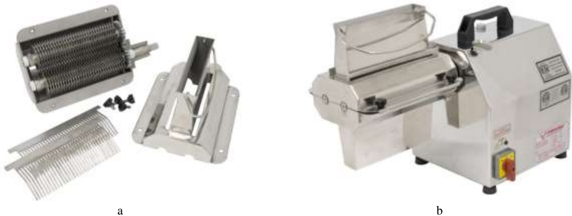
Fig. 2. A table-top rotary tenderizer by American Eagle Food Machinery [12]
